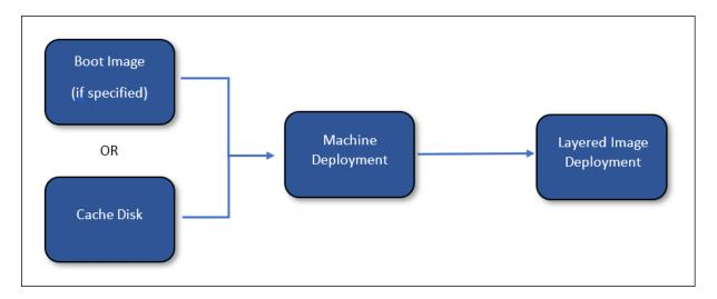
If a **Layered Image** deployment is specified, then the resources created by the **Machine** deployment are deleted after the **Layered Image** deployment completes. Otherwise, App Layering does not delete the resources (unless the deployment fails).
