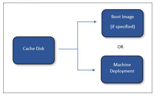
If a **Boot Image** deployment is specified, then the resources created by the **Cache Disk** deployment are deleted after the **Boot Image** deployment completes. Otherwise, App Layering deletes the resources during cache cleanup.
