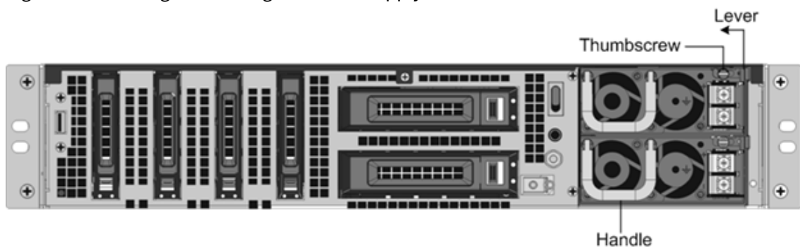
Figure 3. Removing the Existing DC Power Supply
