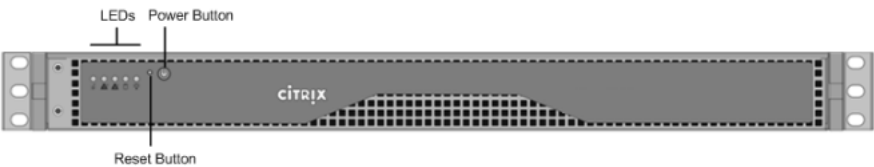
Figure 1. Citrix SD-WAN 1000 PE (EE), front panel
