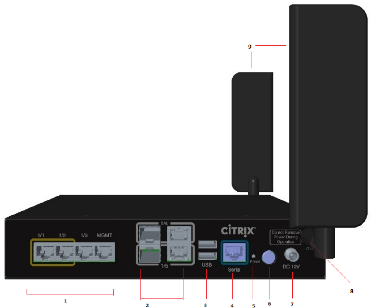
Figure 4. 210 SE (LTE) back panel with antenna
