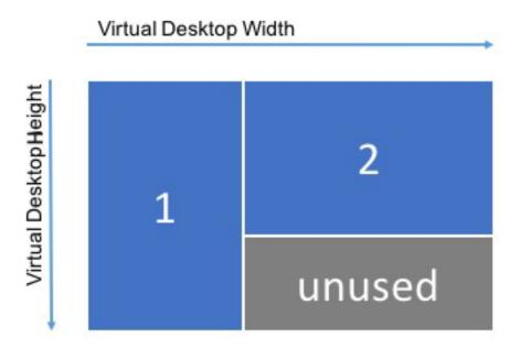
If each monitor in the above diagram has a resolution of 2560×1600, the out-of-the-box multi-monitor configuration parameters are insufficient. The maximum height is too small to accommodate the virtual session desktop for this monitor layout. To accommodate the client monitor configuration in this example, you must set the macOS VDA virtual desktop to a size of 4160×2560.
