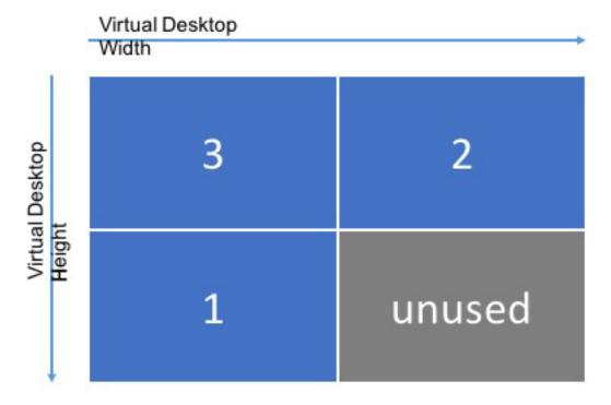
A virtual session desktop size needs to be  $5120 \times 3200$  to accommodate the client monitor configuration if each monitor has a resolution of  $2560 \times 1600$
