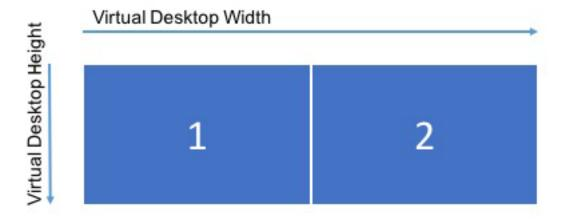
The diagram shows an out-of-the-box multi-monitor configuration with two monitors, each with a resolution of 2560×1600.
