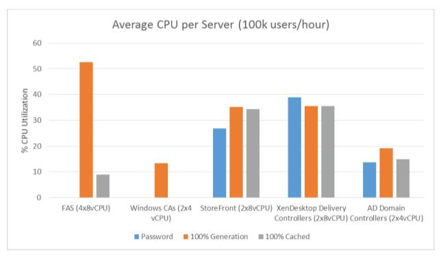
The quantity and CPU configurations of the non-FAS virtual machines are provided for reference and may not match what is required for your environment.
