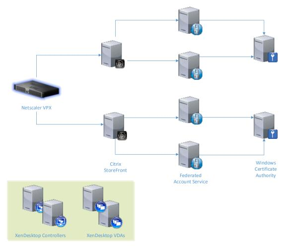
Authentication workflow used for 100,000-user testing
