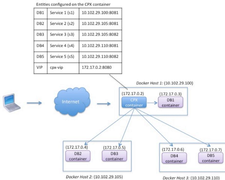
In this example, the NetScaler CPX instance and a server (DB1) are provisioned on the same Docker host with IP address 10.102.29.100. Four other servers (DB2, DB3, DB4, and DB5) are provisioned on two different Docker hosts, 10.102.29.105 and 10.102.29.110.
