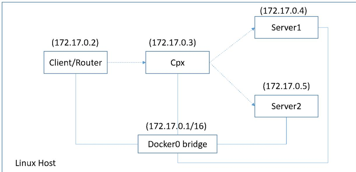
In this topology, virtual servers are configured and advertised (based on the health of services) to the upstream network or router using BGP.
