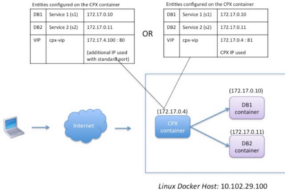
In this example, the NetScaler CPX instance (172.17.0.4) and the two servers, DB1 (172.17.0.10) and DB2 (172.17.0.11) are provisioned on the same Docker host with IP address 10.102.29.100. The client resides elsewhere on the network.
