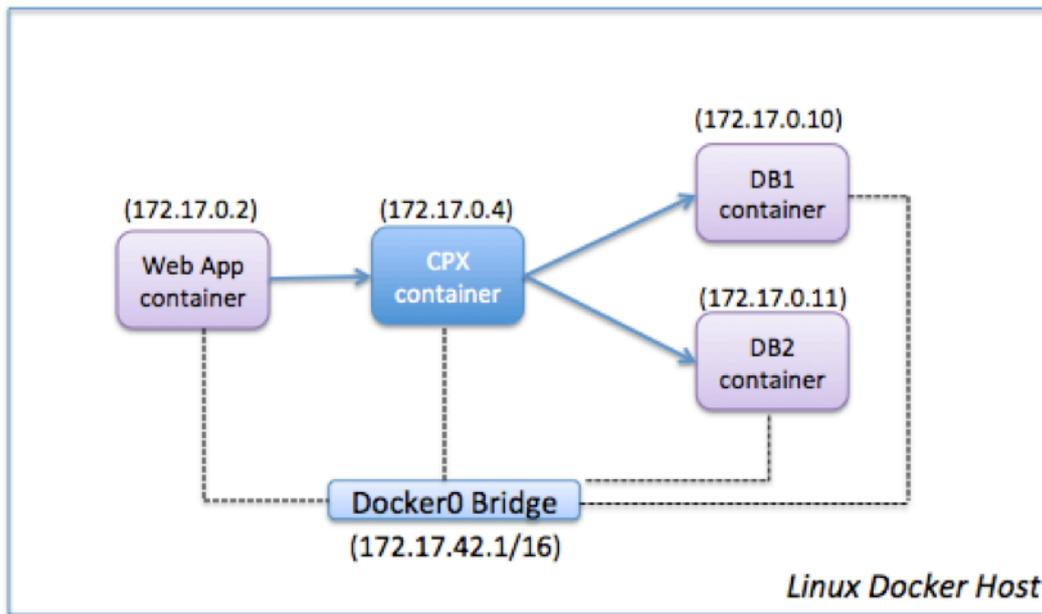
In this example, a web app container (172.17.0.2) is the client and the two database containers, DB1 (172.17.0.10) and DB2 (172.17.0.11), are the servers. The NetScaler CPX container (172.17.0.4) sits between the client and the servers acting as a proxy.
