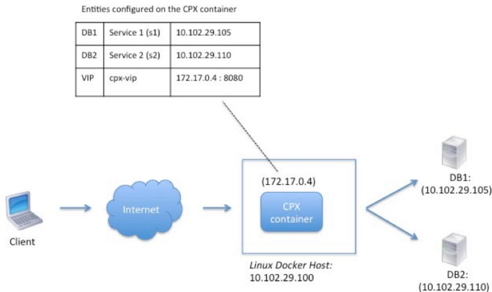
In this example, the NetScaler CPX container (172.17.0.4) sits between the client and the physical servers acting as a proxy. The servers, DB1 (10.102.29.105) and DB2 (10.102.29.110), reside outside a Docker host on the network. The client request originates from the Internet and is received on the NetScaler CPX, which distributes it across the two servers.
