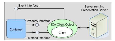
This diagram outlines the interfaces between the ICA Client Object and the container.
