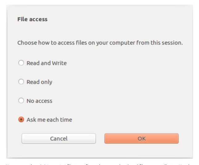
You can use the wfclient.ini file to configure the mapped path and file name attributes. Use the GUI to set a file access level as shown in the preceding screen capture.
