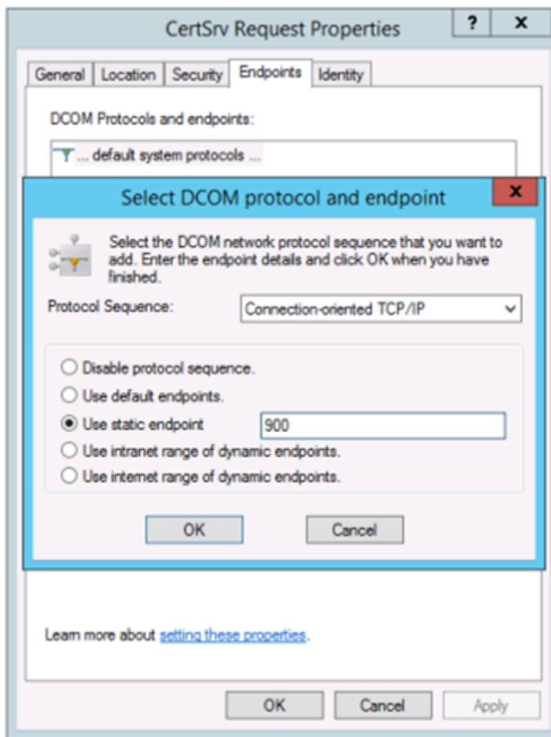
Change the “Endpoints” to select a static endpoint and specify a TCP port number (900 in the graphic above).
