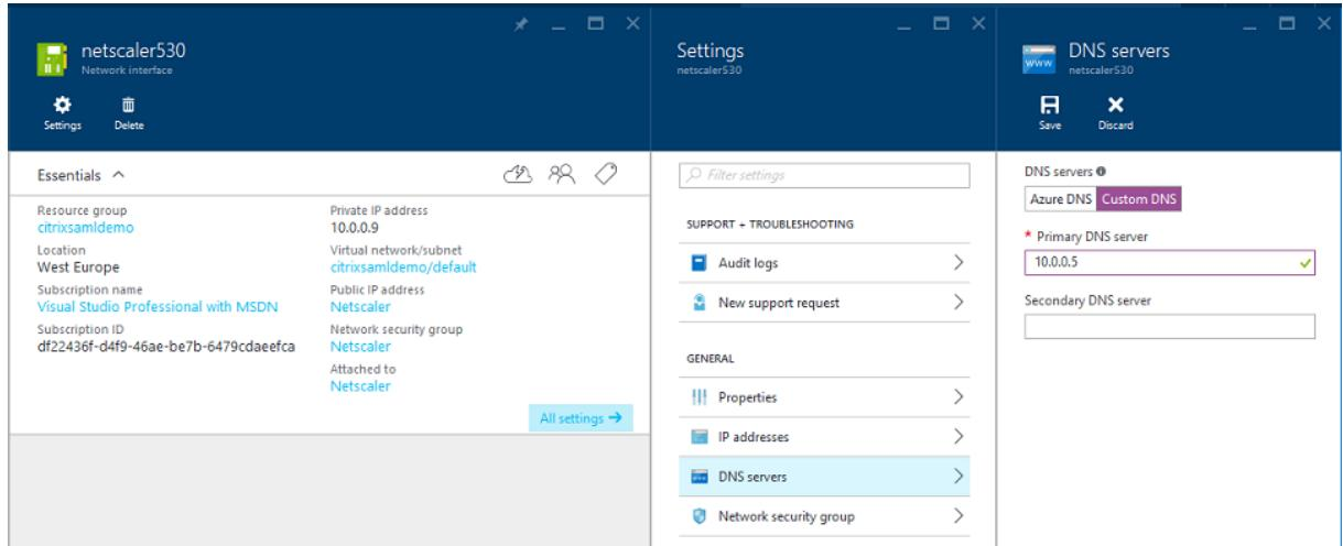
By default, the internal IP (10.0.0.9) address is dynamically allocated. You can use the IP addresses setting to permanently assign the IP address. This should be done for the Web Application Proxy server and the domain controller.
