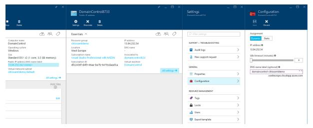
This example assigns a DNS address of domain control-citrix samldemo. westeurope. cloud app. azure. com to the domain controller.
