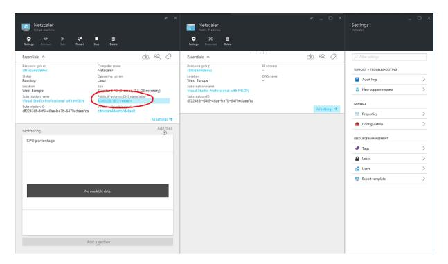
Select **Configuration** of the **Public IP address/DNS name label**. Choose a public DNS address for the VM. This can be used for CNAME references in other DNS zone files, ensuring that all DNS records remain correctly pointing to the VM, even if the IP address is reallocated.
