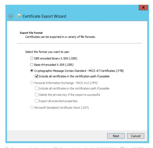
The format must be "Cryptographic Message Syntax Standard – PKCS #7 Certificates (.P7B)" and "Include all certificates in the certification path if possible" must be selected.
