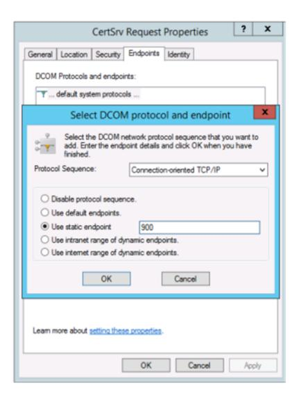
Change the **Endpoints** to select a static endpoint and specify a TCP port number (900 in the preceding graphic).
