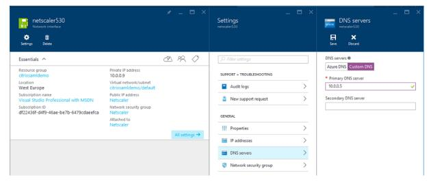
By default, the internal IP (10.0.0.9) address is dynamically allocated. You can use the IP addresses setting to permanently assign the IP address. This should be done for the Web Application Proxy server and the domain controller.
