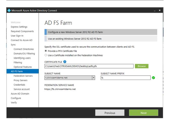
When prompted to select a proxy server, enter the address of the wap.citrixsamldemo.net server. You may need to run the **Enable-PSRemoting –Force** cmdlet as an administrator on the Web Application Proxy server, so that Azure AD Connect can configure it.
