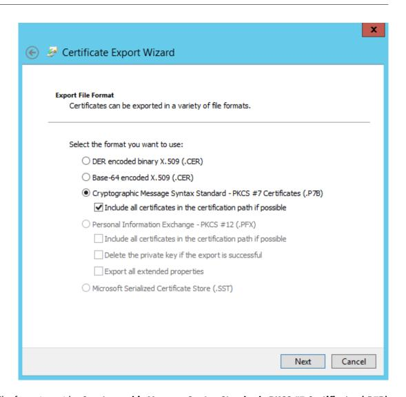
The format must be **Cryptographic Message Syntax Standard –PKCS #7 Certificates (.P7B)** and **Include all certificates in the certification path if possible** must be selected.
