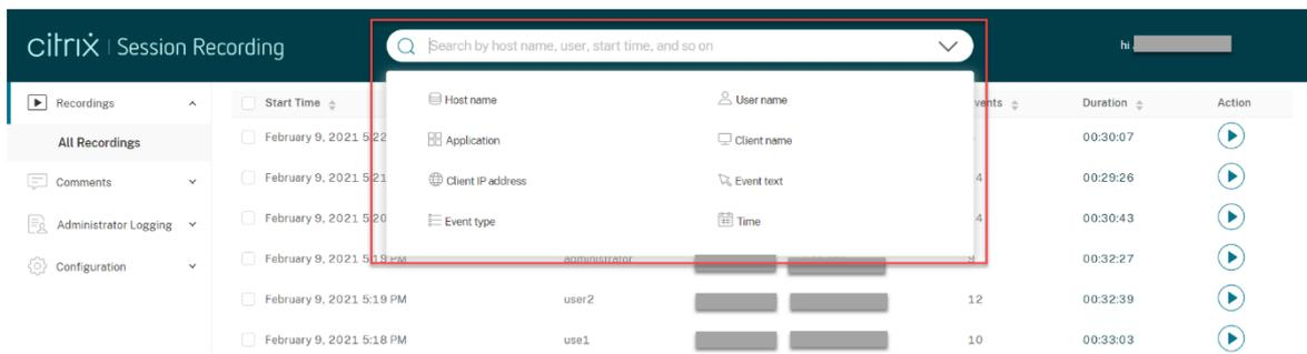
For example, after you select the host name filter, the following dialog box appears. Type in the host name (of the VDA where recorded sessions are hosted) and click **Search** to filter out irrelevant recordings and display only the relevant ones.
