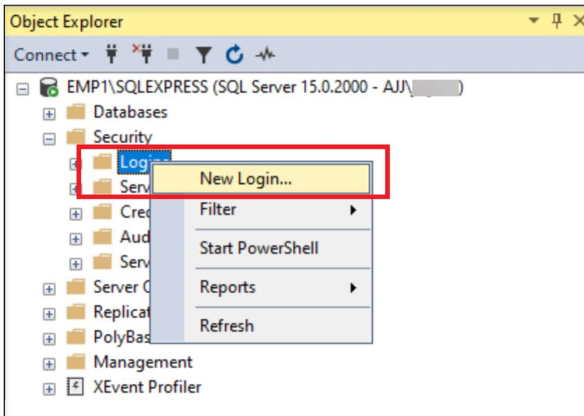
Name the new login in the format of **<domain name of the domain controller>\<name of the gMSA>**. For example:
