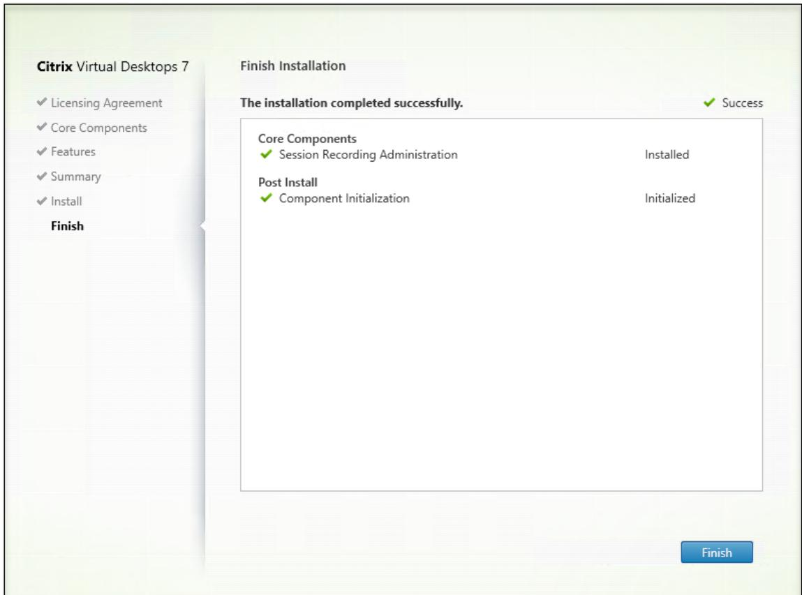
The **Finish Installation** page shows green check marks for all the prerequisites and components that have been installed and initialized successfully.
