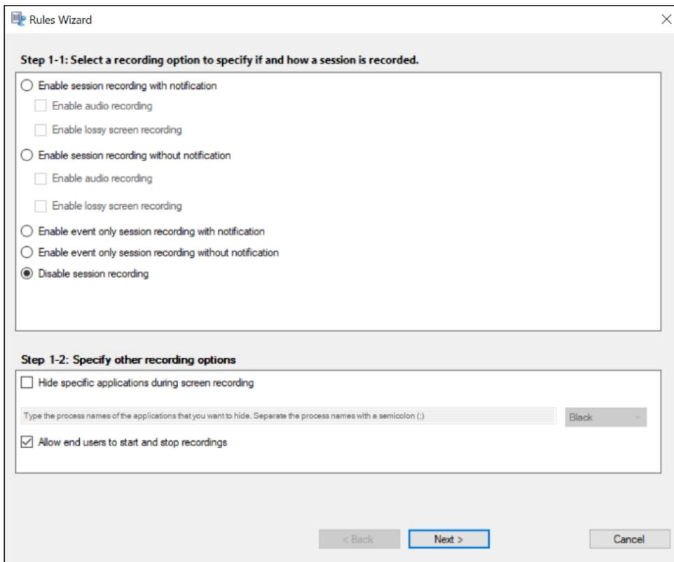
When you select **Enable session recording with notification** or **Enable session recording without notification**, you can further select to enable audio recording or lossy screen recording.
