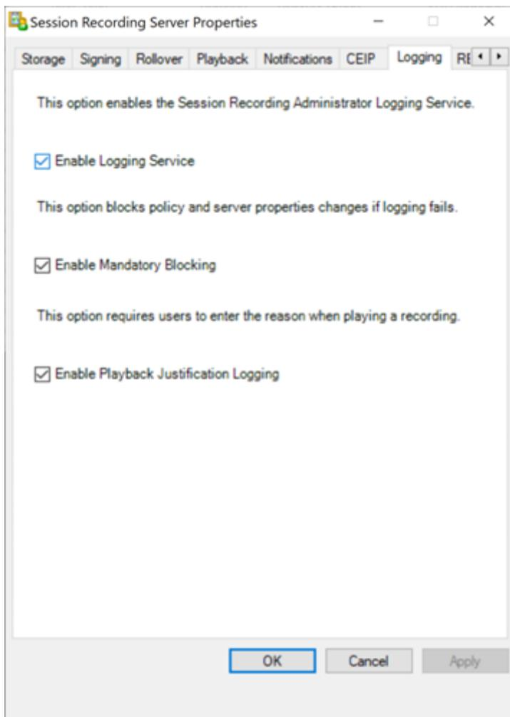
With playback justification logging enabled, each time you play a recording, a dialog box appears, asking you to enter a playback justification. For example, see the following screen captures:
