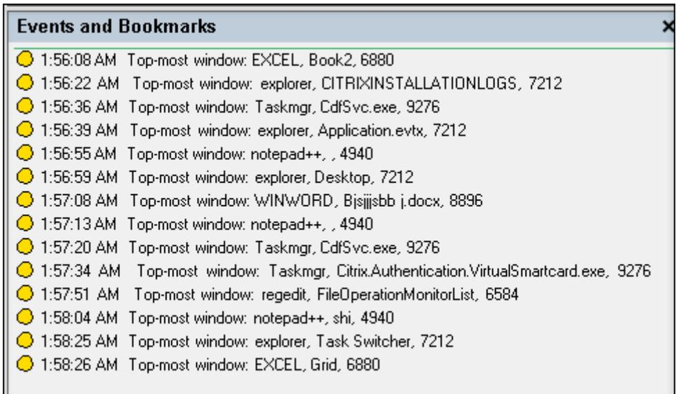
**Clipboard activities** Session Recording can detect copy operations of text, images, and files using the clipboard. The process name and file path are logged for a file copy. The process name and title are logged for a text copy. The process name is logged for an image copy.
