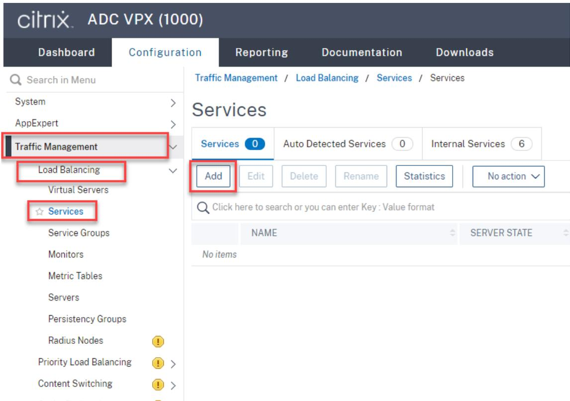
**(Required only when you are using the WebSocket server Version 1.0) Add an SSL load balancing service of port 22334 for each Session Recording server.** Type a name for the load balancing service, choose **Existing Server**, select the IP address of a Session Recording server, select **SSL** as the server protocol, type port number **22334**, and click **OK**.
