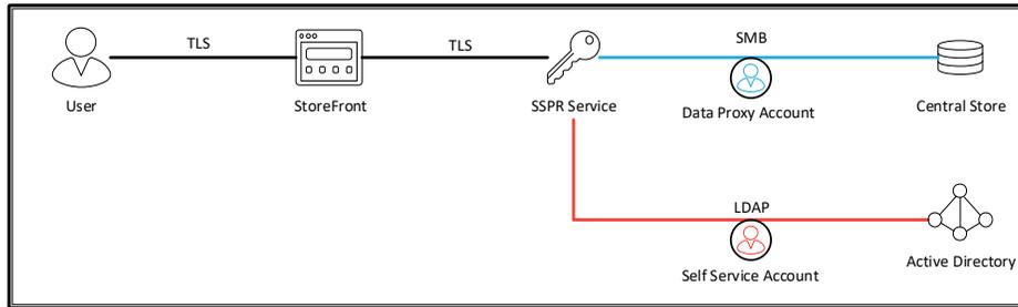
Figure 24: SSPR Architecture
