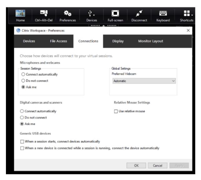
The two check boxes at the bottom of the pane controls if the devices must connect automatically or wait for manual connection in the session. These settings are not enabled by default. You can change the preferences if generic USB devices must be connected automatically.
