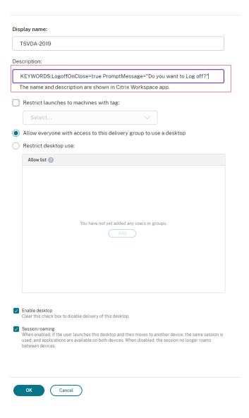
The keywords are assigned by default for new desktop machines assigned to the group. For existing desktop machines, you must run the following powershell commands for changes to apply:
